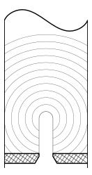
Notice the shallow hole in the bottom of the rocket engine. This is where the igniter is inserted and ignites the fuel (a substance similar to black powder or gun powder, only packed and bound into a cylindrical solid). The fuel starts burning at the ignition point and spreads from there in a uniform way.
