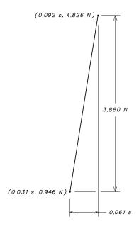
From the diagram we can see that for this section of the curve, 3.880 Newtons is proportional to 0.061 seconds, so that we can find the slope M as the ratio 3.880 N/0.061 s or approximately 63.607 N/s. M is a sort of conversion<sup>8</sup> from seconds to Newtons for this specific line segment. Before we move on to the intercept,
