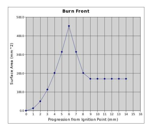
Recall the reasoning that the surface area of the burn is proportional to the engine thrust and suddenly you are looking at the rough shape (an estimate using our simplistic theoretical model) of the engine **thrust profile**! It isn't nearly the constnat engine thrust profile we used in our trajectory calculations of the previous chapters. Furthermore, as the fuel burns, the engine mass decreases and further affects the trajectory calculations.
